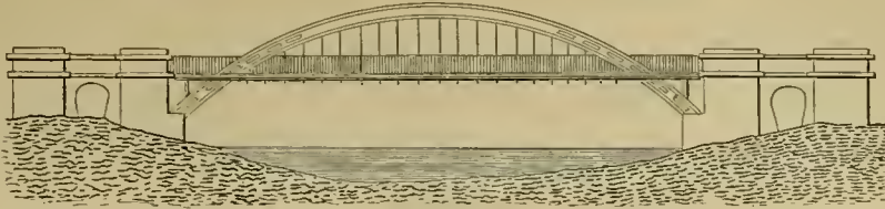
Bow-String Bridge at Howeslett, England.
